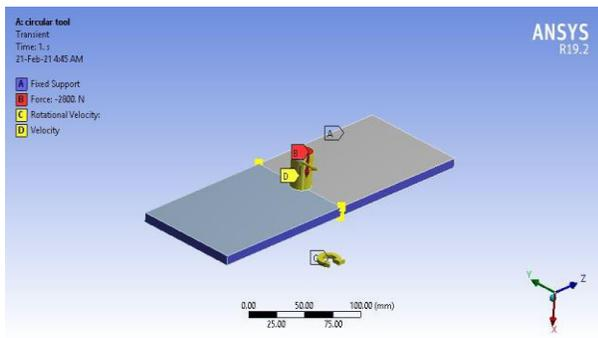
Here boundary conditions applied with an RPM of 900 and the force of spindle assume to be 2800N and required axial velocity
