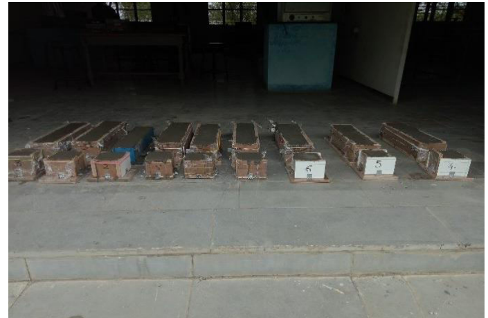
Fig 14:- 9 cubes and 9 prisms were casted with M20 concrete mix
