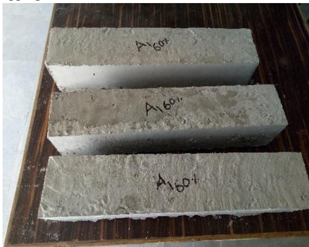
Fig 18: - 3 prisms casted with AGE 1 recycled coarse aggregate (R.C.A) with 60% replacement of natural coarse aggregate (N.C.A)
