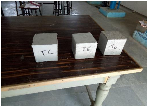
Fig 12:- 3 cubes which were casted with traditional concrete
