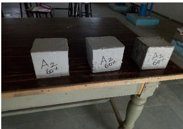
Fig 24: - 3 cubes casted with AGE 2 recycled coarse aggregate (R.C.A) with
