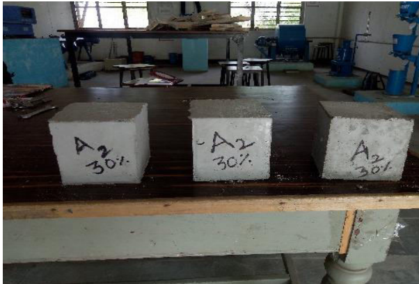
Fig 22:- 3 cubes casted with AGE 2 recycled coarse aggregate (R.C.A) with 30% replacement of natural coarse aggregate (N.C.A)
