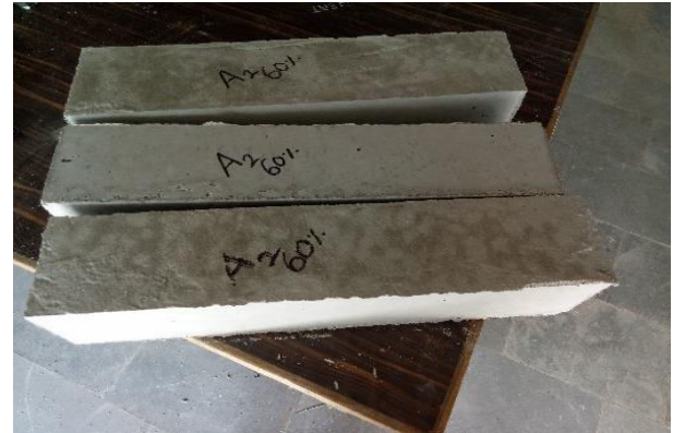
Fig 25: - 3 prisms casted with AGE 2 recycled coarse aggregate (R.C.A) with 60% replacement of natural coarse aggregate (N.C.A)
