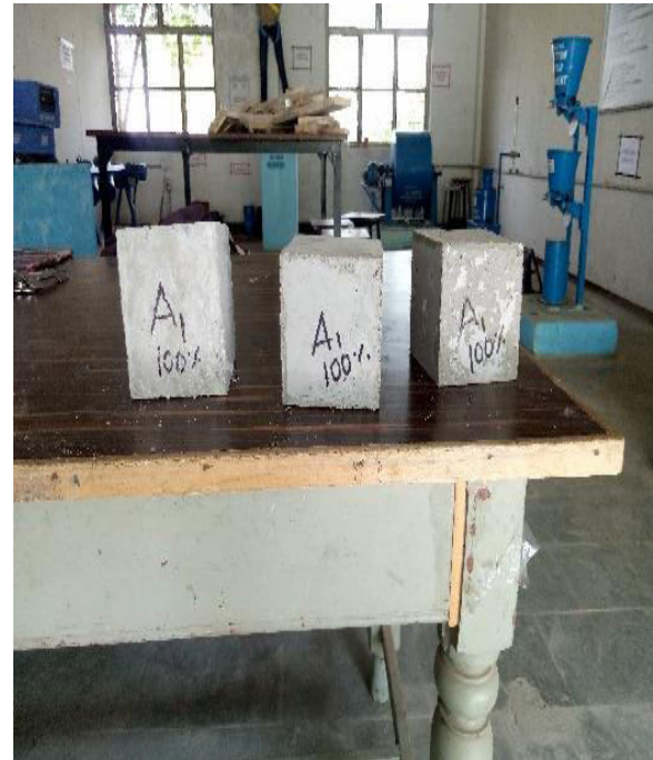
Fig 19: - 3 cubes casted with AGE 1 recycled coarse aggregate (R.C.A) with 100% replacement of natural coarse aggregate (N.C.A)
