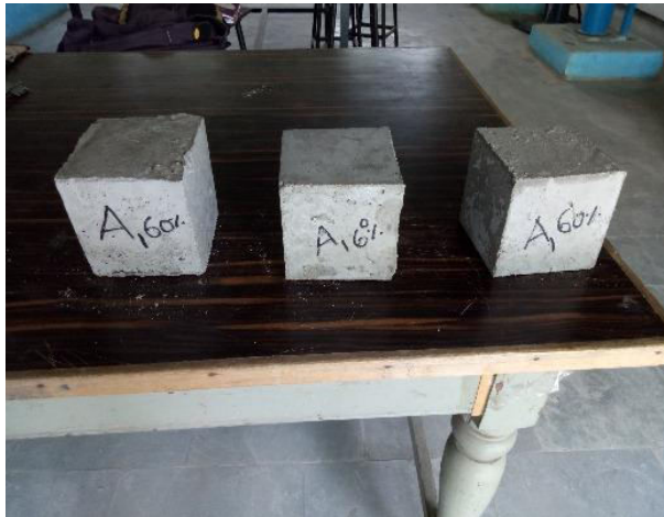
Fig 17: - 3 cubes casted with AGE 1 recycled coarse aggregate (R.C.A) with 60% replacement of natural coarse aggregate (N.C.A)
