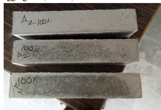
Fig 27: - 3 prisms casted with AGE 2 recycled coarse aggregate (R.C.A) with 100% replacement of natural coarse aggregate (N.C.A)
