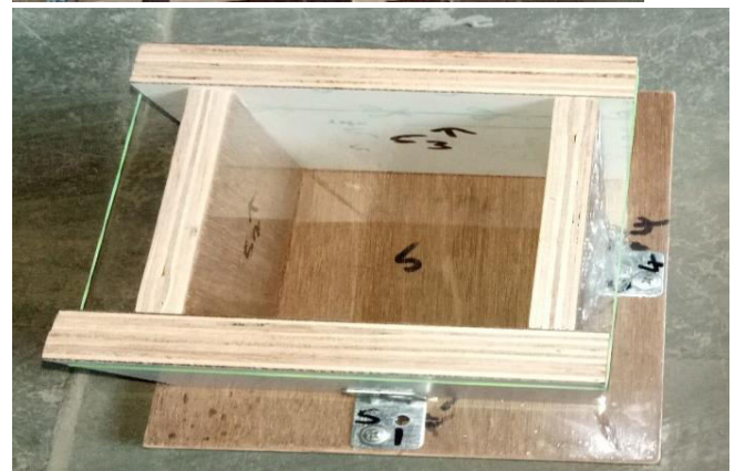
Fig 11 :- Moulds in which concrete has to be caste
