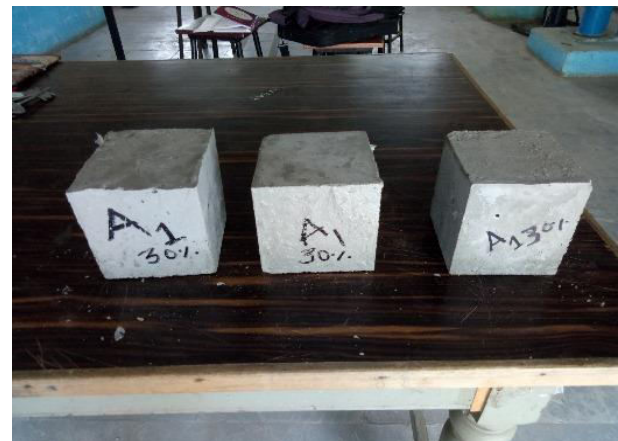
Fig 15: - 3 cubes casted with AGE 1 recycled coarse aggregate (R.C.A) with 30% substitution of natural coarse aggregate (N.C.A)
