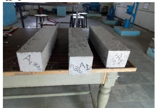
Fig 16: - 3 prisms casted with AGE 1 recycled coarse aggregate (R.C.A) with 30% replacement of natural coarse aggregate (N.C.A)
