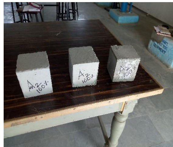
Fig 26: - 3 cubes casted with AGE 2 recycled coarse aggregate (R.C.A) with 100% replacement of natural coarse aggregate (N.C.A)
