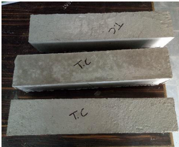
Fig13: - 3 prisms were casted with traditional concrete
