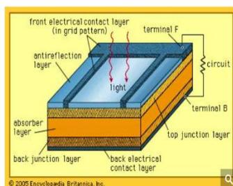
Diagram of a solar cell structure
