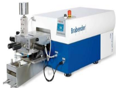
Figure 6 Brabender internal melt blending mixer
