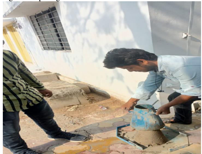
Fig.8: Checking the Slump Value at the Laboratory
