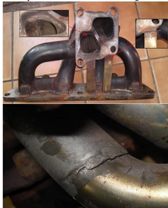
Fig: Defects in End connections due to thermal stress
