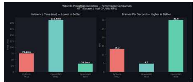
Figure 4.4.3 Comparison of YOLOv8 Performance Using PyTorch FP32, OpenVINO FP32, and OpenVINO INT8 in Terms of Inference Time (ms) and Frames Per Second (FPS) on CPU
