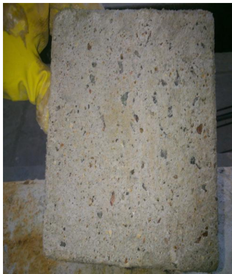
Figure 14. Visual observation of cube removing from 5% HCL
