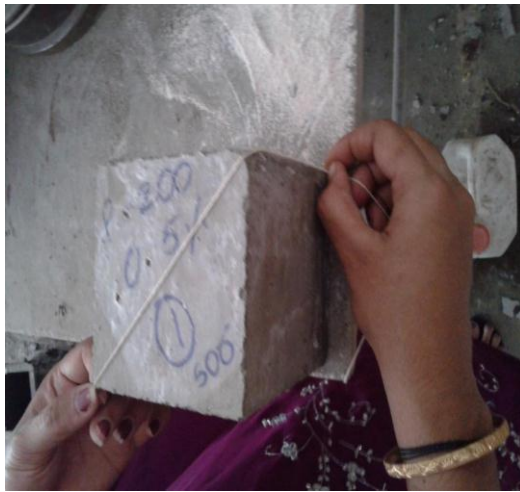
Figure 10. Measuring diagonal dimension of cube
