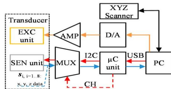
**Figure 4: The utilized measuring system configuration diagram.**
