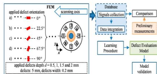
**Figure 5: The Finite Element Method to defect the Measurement Model.**
