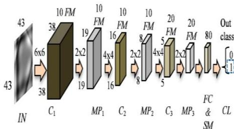
**Figure 3: Schematic view of the deep convolutional neural network (DCNNDND) architecture for evaluation of defect occurrence;**
