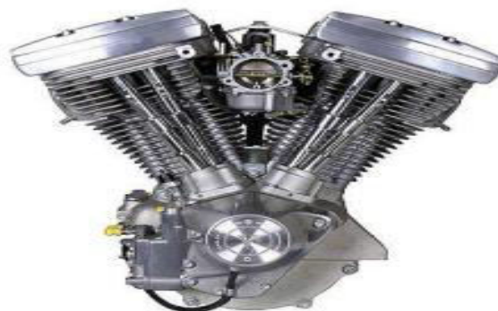
Figure: Air cooling system
