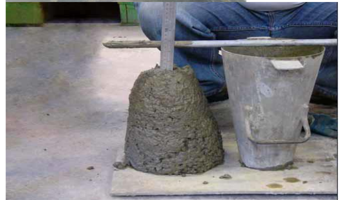
111 FIG :5.8SLUMP CONE TYPICAL SLUMP CONE
