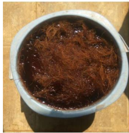
Fig.3.12: Oil immersion of coconut fiber
