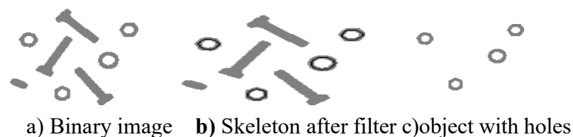
Figure 4: Isolation of objects with holes using morphological operations.
