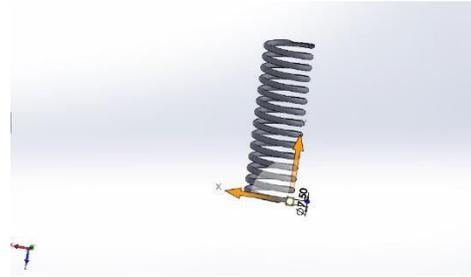
15.5mm helix pitch with 7.5mm coil diameter
