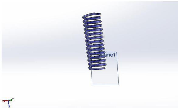
15mm helix pitch with 8mm coil diameter
