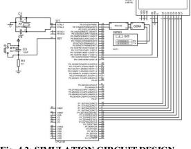
Fig. 4.2: SIMULATION CIRCUIT DESIGN WITH GSM AND GPS INTERFACE
