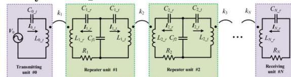
**Fig. 2: SPS STRUCTURE OF MULTI-LOAD WPT REPEATER SYSTEM**
