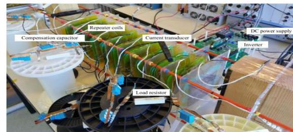
Fig. 5: EXPERIMENTAL SETUP WITH SPS COMPANSETION TOPOLOGY
