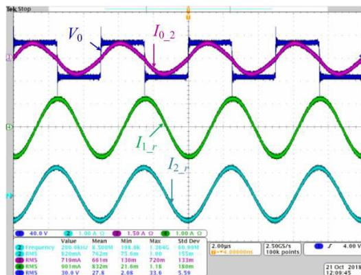
**Fig. 7: EXPERIMENTAL LOAD WAVEFORMS OF WITH SPC COMPANSETION TOPOLOGY**
