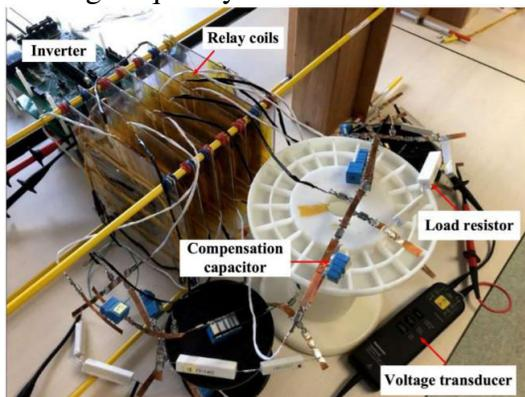
Fig. 4: EXPERIMENTAL SETUP WITH LCC COMPANSETION TOPOLOGY
