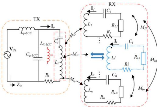
**Fig. 3: LLC STRUCTURE OF MULTI-LOAD WPT REPEATER SYSTEM**
