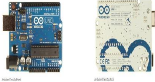
Fig 2: Arduino (TM) UNO Rev 3 Board. Specifications:
