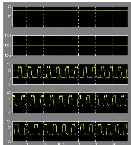
Fig 10 Simulation waveforms of the proposed method torque (Te),Speed (Wr), Load Currents (Iabc)
