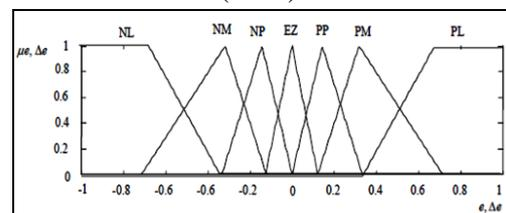
Fig.7 Membership functions for Input, Change in input, Output.
