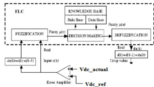
Fig.6. Block diagram of the Fuzzy Logic Controller (FLC).
