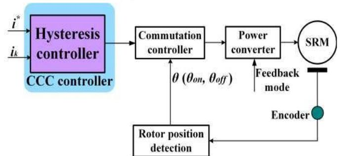
Fig 3 Control strategy under regenerative braking modes
