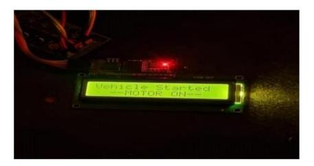
If the fingerprint is verified as non-authorized, then motor does not gets started and "INVALID FINGER MOTOR OFF" will be displayed on the LCD.
