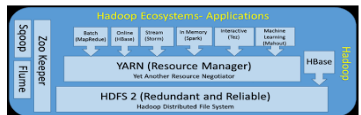
Fig 2. The image shows the Hadoop technology stack. Hadoop core/common which consists of HDFS which is a programmable interface to access stored data in cluster.
