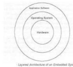
Fig 2 overview of embedded system architecture
