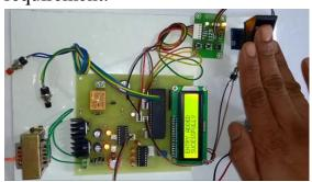
The finger print scanner serves as the main input into this embedded security system. Finger prints read are compared to those ones preprogrammed into the memory of the microcontroller. When a match is made, the microcontroller outputs a HIGH which activates the transistor-relay switching stage that controls opening and closing of the modelled motorized door granting access into the protected building. An
