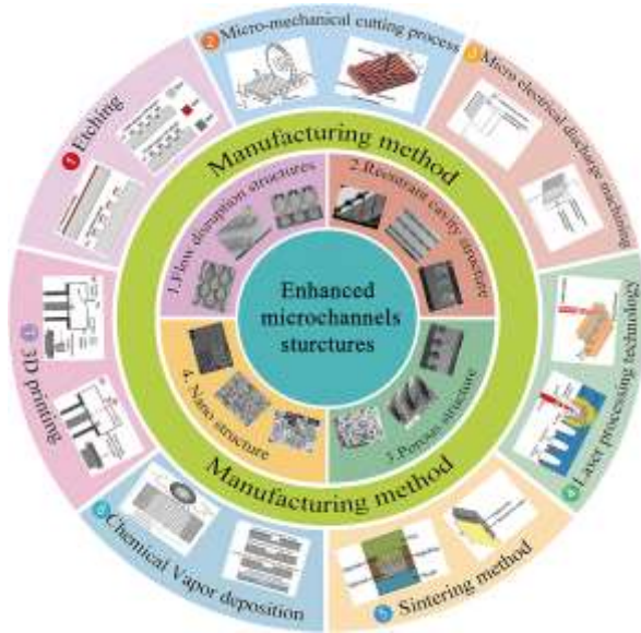
Figure 1 Summary of Enhanced microchannels structures and their fabrication method [15] (Deng et.al 2021)
