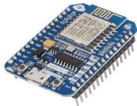
Figure 2 :NodeMCU Development Board/kit v0.9 (Version1)
