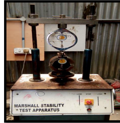
Figure.3 Marshall stability test setup
