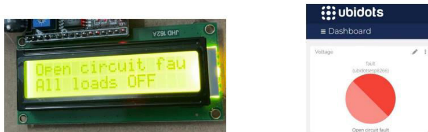
Figure 3. Open circuit fault
