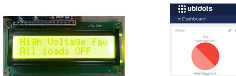
Figure 4. High voltage fault
