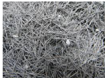
Figureno.3.2 Waste steel fibres
