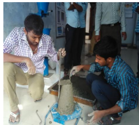
Fig.3 Slump Cone test
