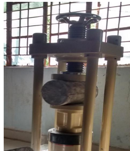
Fig.5: Split tensile sample testing
