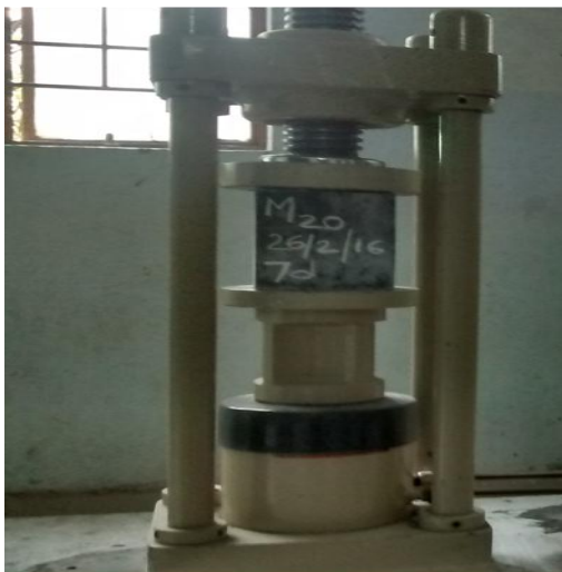
Fig.4 Compressive strength testing machine
