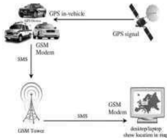
Figure 1 Architectural View of Anti-Theft Vehicle Tracking System
