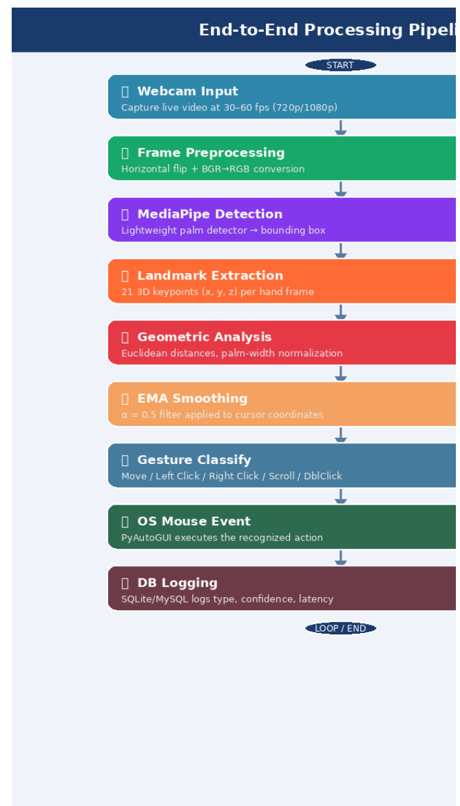
Figure 1: End-to-End Processing Pipeline (Webcam → Gesture → OS Action)
