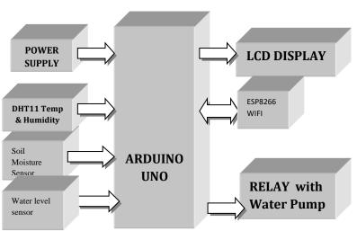
The design and development of a smart monitoring and controlling system for agriculture environment in real time has been reported. The system principally monitors parameters such as temperature, moisture level, humidity and water level of the agriculture field. Users can monitor and control transducers on active The system offers a complete, low cost, powerful and user-friendly way of real-time monitoring and remote control of field.
