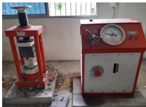
Fig. 7: Compressive Strength test of cube sample.
