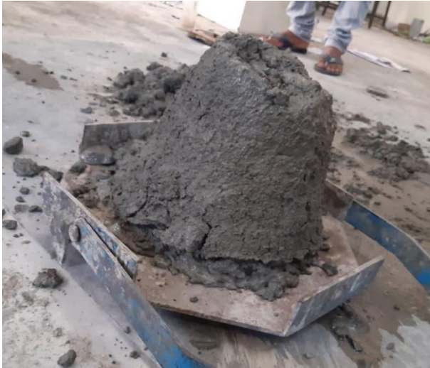
Fig. 6: Slump cone test.
