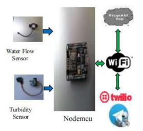
Figure 1 illustrates the block diagram of the water pipeline leakage detection system. The NodeMCU is a cost-effective Wi-Fi microcontroller featuring 8 digital pins and one analog input pin, with all pins supporting interrupts except for D0. The
