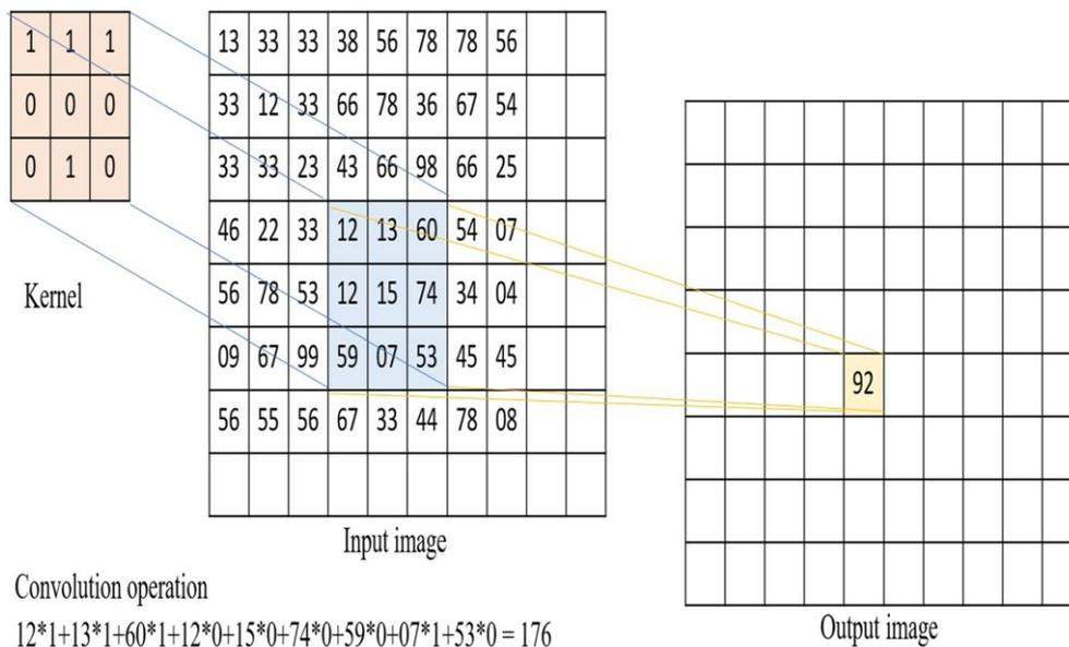
Fig. 2 The Convolution filter operation is done with  $3 \times 3$  kernel. Each pixel from input image and its eight of the neighboring pixels are multiplied with corresponding value in kernel matrix, and then finally, all multiplied values are added to achieve the final output .
