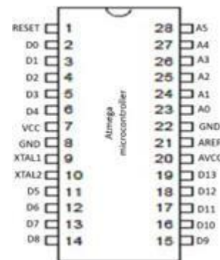
Fig.3. Schematic Diagram of Atmega microcontroller
