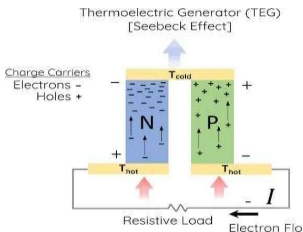
In this method we used thermoelectric generator for generating electric generator
