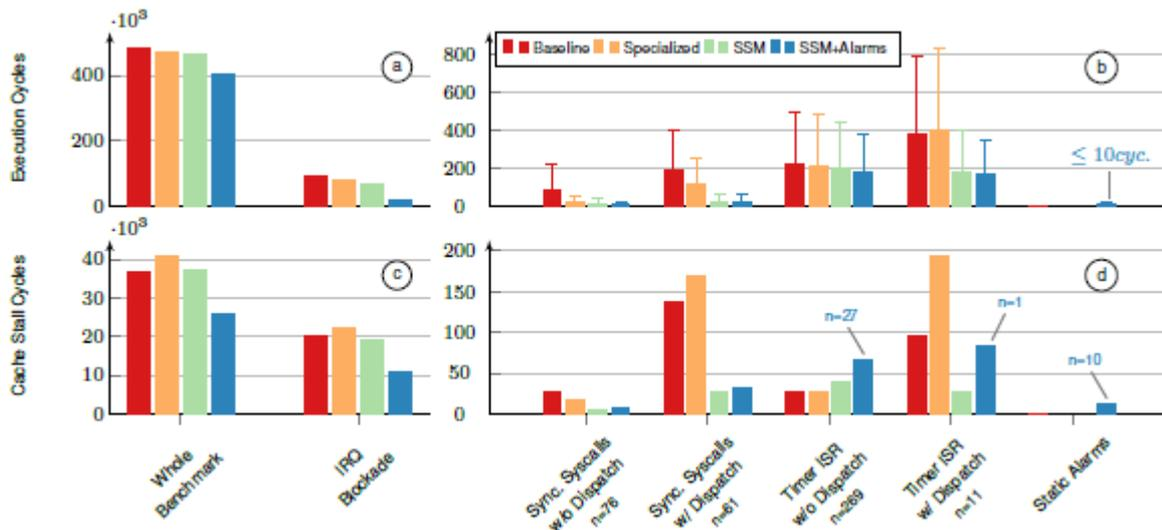
Figure 7: Results for I4Copter in the Cycle-Accurate Simulator generated by the Rocket Toolchain. at least a 75 percent benefit over the baseline, while the average benefit is even over 90 percent.
