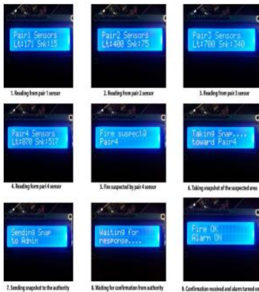
Fig. 8. Sensor reading, taking and sending snap, authentication and fire status displaying in LED.
