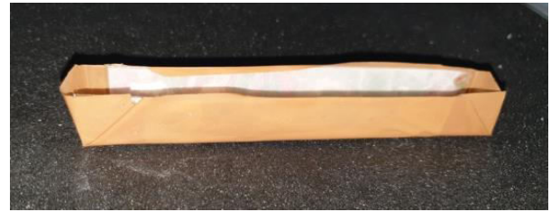
Fig-4: Mould for tensile and bending test
