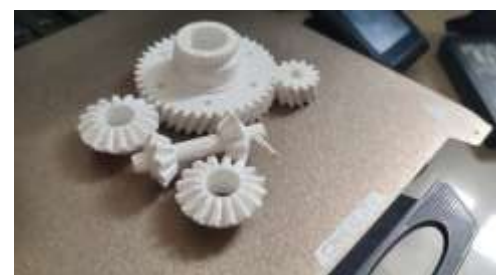
Fig 3.11 Printing of Gears
