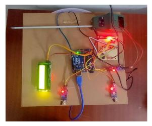
We have prosposed a digital fuel meter with fraud detection. We have used ultrasonic sensor for measuring the volume in the container. We used the pH senor for measuring the pH of the fuel. The fuel when mixed with water, the pH changes accordingly.
