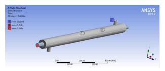
Static structural → supports → fixed support → inlet outlet areas
