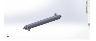
Double pipe heat exchanger final assembly model
