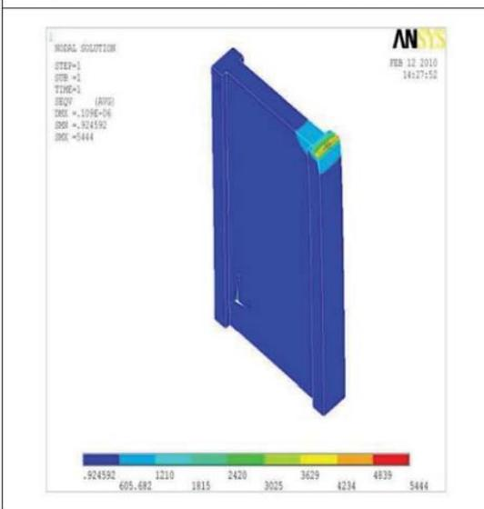
shown in Figures 8 and 9. Von Mises stress contour was shown in Figures 10 and 11 and it was observed that the maximum stress is at the bottom of shear wall. The possibility of modeling the flanged shear wall can be extended for modeling all the reinforced structures under lateral cyclic loading.
