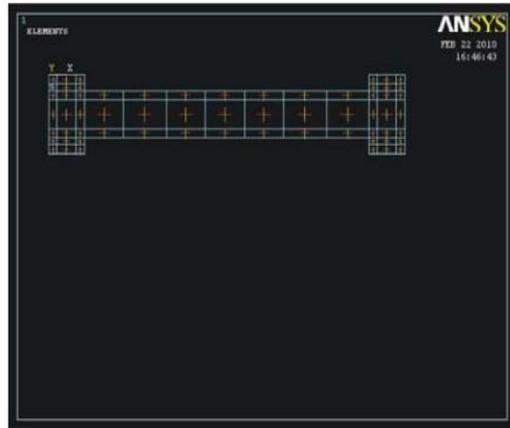
**Figure 6: Shear Wall with Smeared Reinforcement**
