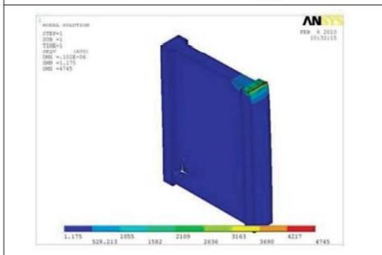
**Figure 11: VonMises Stress for Shear Wall With Smeared Model Reinforcement Under Static Loading**
