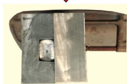
Solidified hybrid (Cu + BaC + MoS 2 ) composite plate
