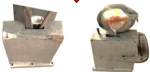
Pouring of the melt mixture into the mould
