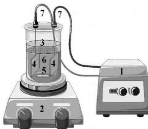
Fig. 1.1: The electrochemical reactor in the laboratory experiments. (1) DC power supply, (2) magnetic stirrer, (3) cover, (4) electrodes, (5) magnetic bar-stirrer, (6) wastewater and (7) electric wire
