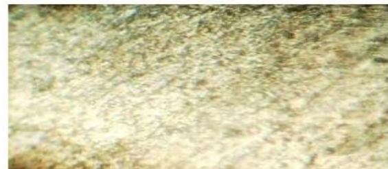
Fig: 14) Optical micro structure of LM 25 Aluminum
