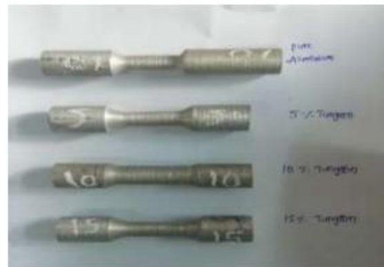
Fig. 8) Machined specimens on Lath
