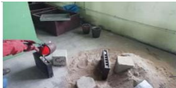
Fig: 2) Poured Liquid metal into mould
