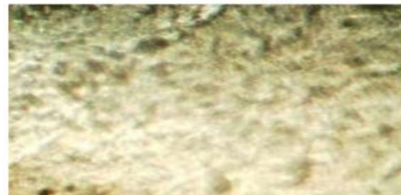
Fig: 15) Optical micro structure of LM 25 Al -5% WC
