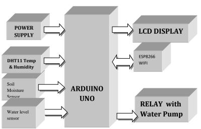
The design and development of a smart monitoring and controlling system for agriculture environment in real time has been reported. The system principally monitors parameters such as temperature, moisture level, humidity and water level of the agriculture field. Users can monitor and control transducers on active The system offers a complete, low cost,
