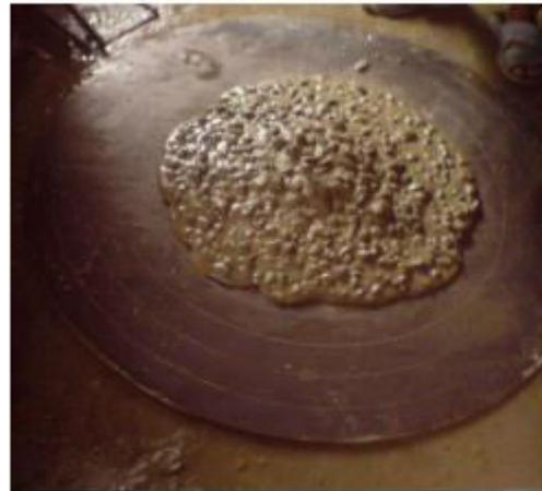
Fig – 6 A photo shown slump value
