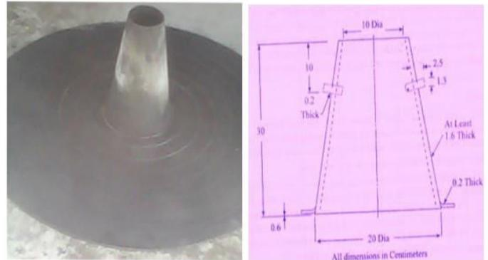
Fig 4 & 5 - Slump cone with dimensions
