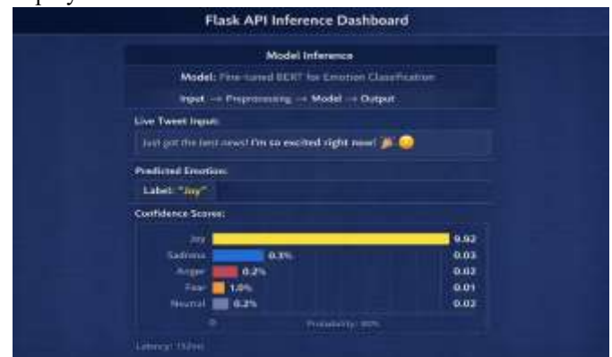
Fig 4.4.2 Flask API Inference Dashboard showing live tweet input, predicted emotion label, and per-class confidence scores returned as JSON.
