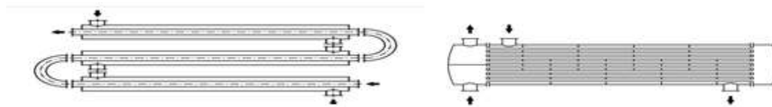
Figure 1: Countercurrent double-pipe heat exchanger Figure 1.1: Segmentally baffled one-pass shell and two-pass tube shell-and-tube heat exchanger
